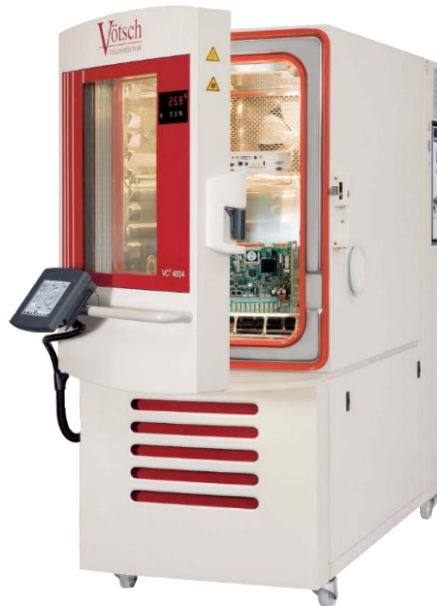
Figure 6: Picture of a Vötsch VT3 4034 Temperature and climatic test system [8], the most commonly model used by BorgWarner in Landskrona.
